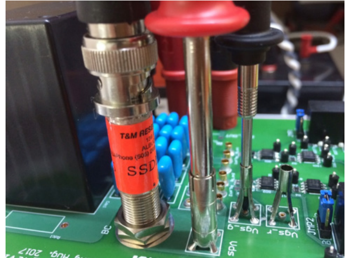
Figure 8: Probe-tip to PCB interface connections
